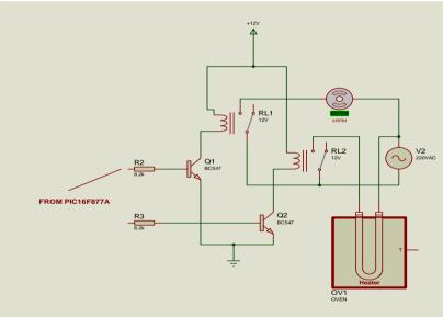
Fig. 6. Switching circuit interfaced to heater and fan
