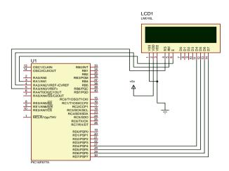
Fig. 5. PIC16F877A and LCD interfacing
