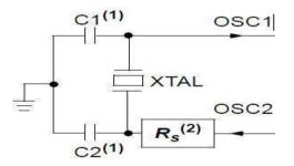
Fig. 4. Crystal oscillator set-up diagram [5]
